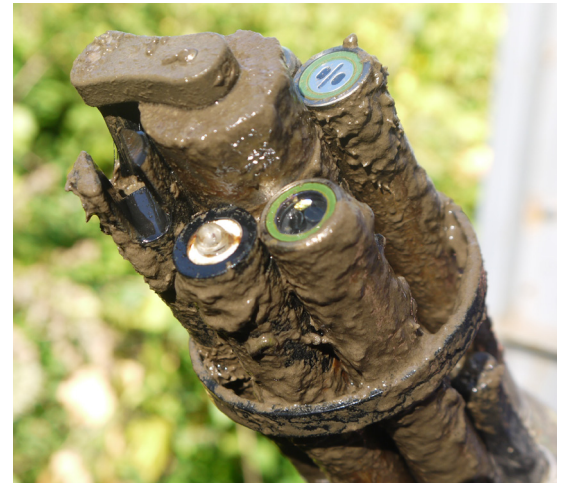
Figure 8. Effective anti-fouling using wiper
